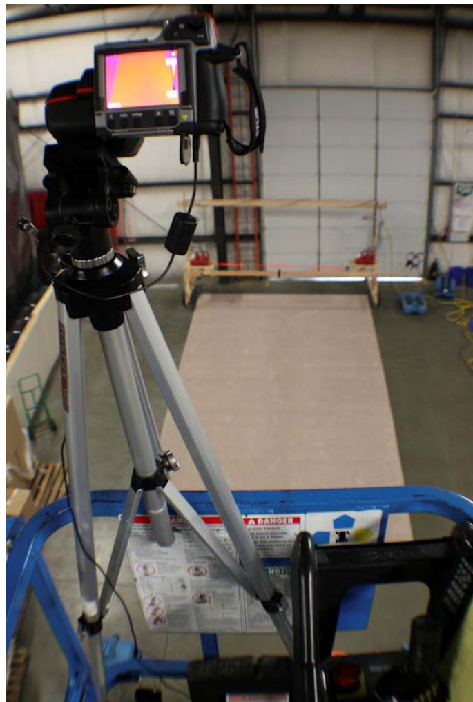
The testing floor as seen from the fixed position thermal imaging camera, located 22 feet above the shop floor
